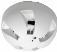
Intelligent thermal with rate of rise and fixed threshold detector for D-Loop with one thermal sensor and a bidirectional isolator for earliest fire detection and indication in all environments with difficult ambient conditions, according to EN 54-5/-17/-18
